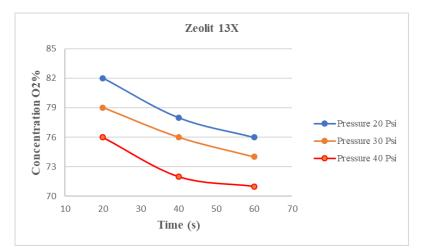
Figure 8. Graph of the effect of pressure on oxygen purity with 13X zeolite
