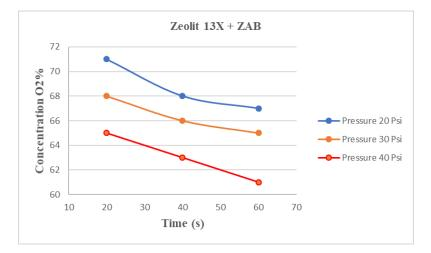
Figure 9. Graph of the effect of pressure on oxygen purity with 13X zeolite + ZAB
