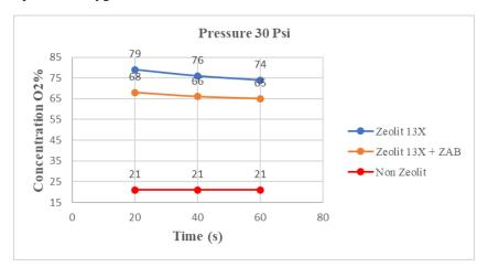
Figure 6. Graph of oxygen purity at the pressure of 30 Psi
