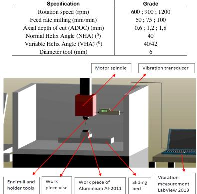
Figure 2. Experimental setup
