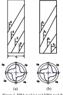
Figure 1. NHA tool (a) and VHA tool (b)
