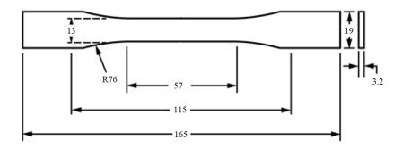
Figure 3: Tensile strength test specimen in millimeter [19].
