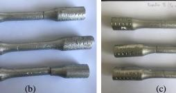
Figure 5. Specimens after tensile test a) 0.12 % wt Fe, b) 0.16 % wt Fe, c) 0.20 % wt Fe
