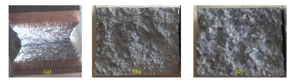
Figure 8. Fracture surface of specimens after impact test a) 0.12 % wt Fe, b) 0.16 % wt Fe, c) 0.20 % wt Fe
