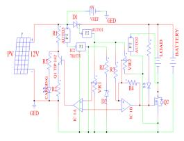
Figure 9. Charge Controller Circuit.
