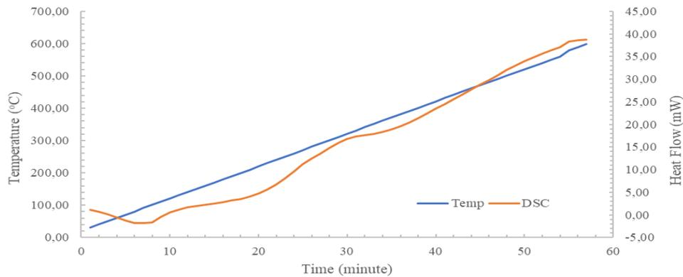
**Figure 10:** DSC curve of DFP + starch 10%.
