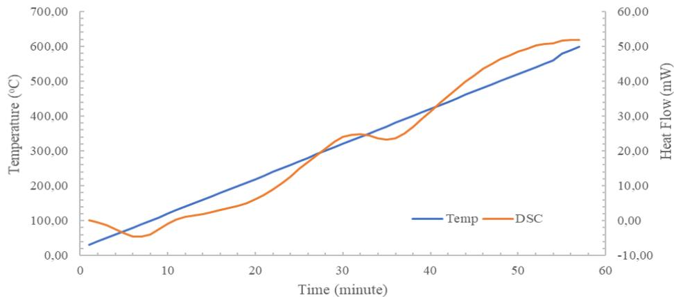
**Figure 11:** DSC curve of DFP + starch 15%.
