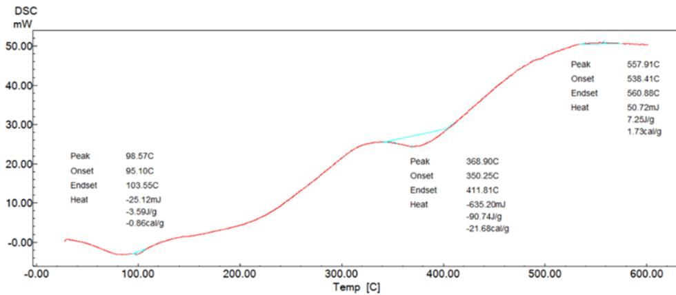
**Figure 6.** DSC thermogram of DFP + starch 10%
