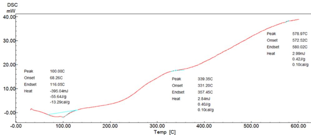
**Figure 4:** DSC thermogram of CS + starch 10%
