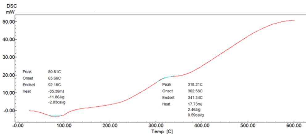
**Figure 5:** DSC thermogram of CS + starch 15%.
