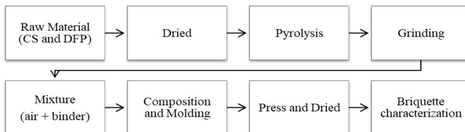
**Figure 2.** Schematic of Briquette Production
