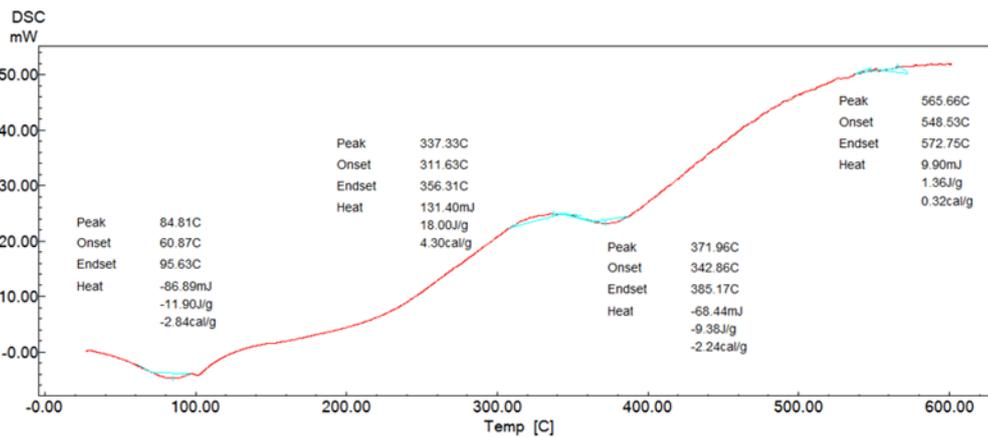
**Figure 7.** DSC thermogram of DFP + starch 15%
