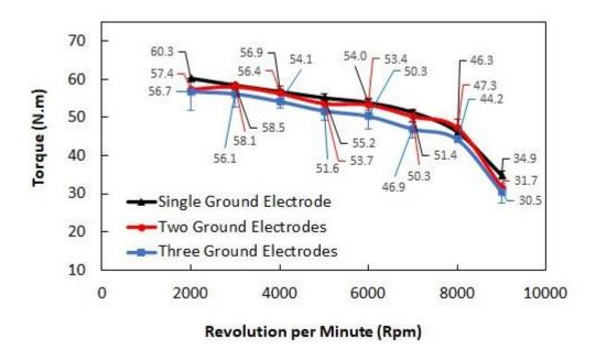
Figure 3. Graph of vehicle Torque as the function of angular velocity on the chassis dynamometer test.
