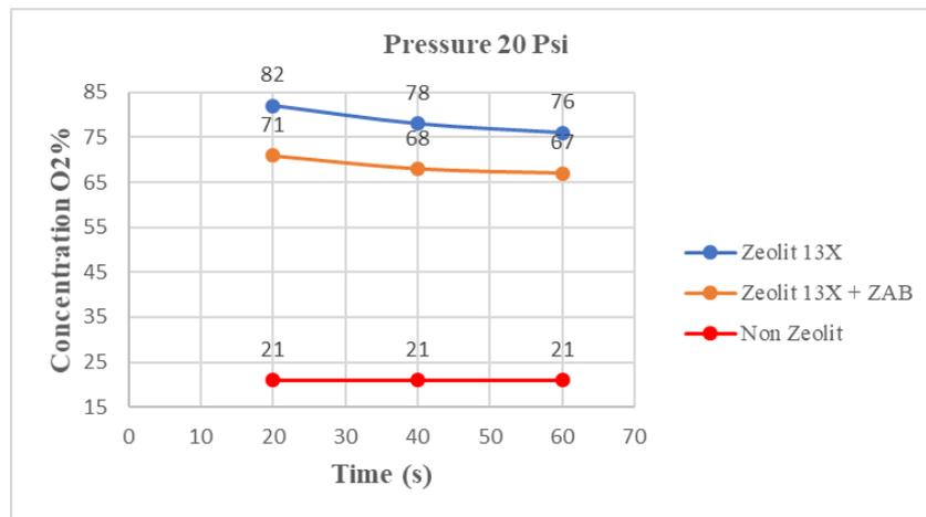
**Figure 5.** Graph of oxygen purity at the pressure of 20 Psi
