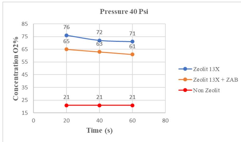
**Figure 7.** Graph of oxygen purity at the pressure of 40 Psi
