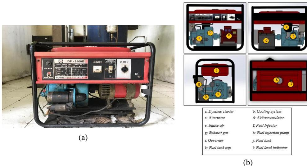
**Figure 1:** (a) Generator type used in this study, (b) Parts of generator components.
