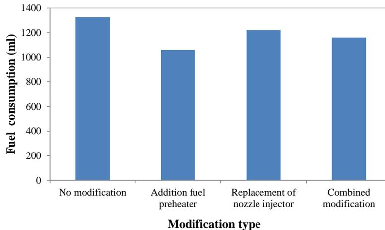
**Figure 2:** The fuel consumption in each engine modification.
