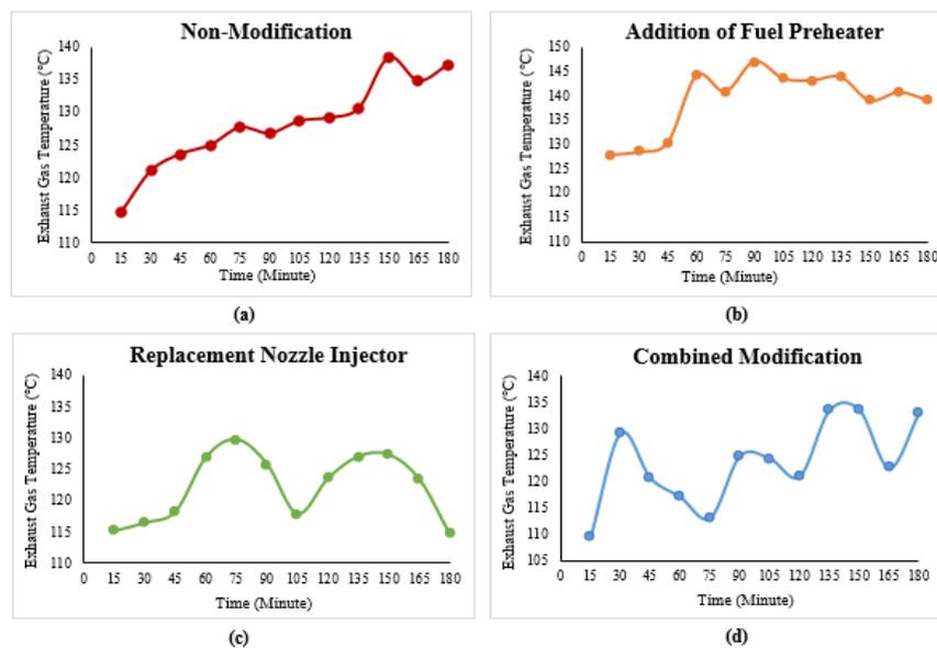
**Figure 5:** (a) Exhaust gas temperature in non-modification, (b) Exhaust gas temperature in addition of fuel preheater, (c) Exhaust gas temperature in replacement nozzle injector, (d) Exhaust gas temperature in combined modification
