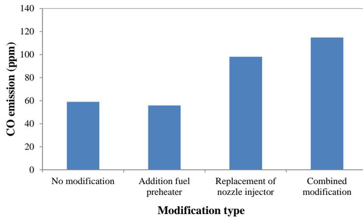
**Figure 3:** The CO emissions in each engine modification.
