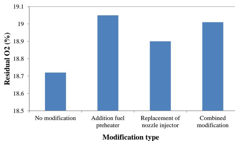
**Figure 4:** The residual O<sub>2</sub> values in each engine modification.
