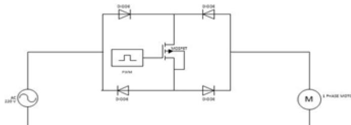
**Figure 2:** Basis AC chopper circuit.
