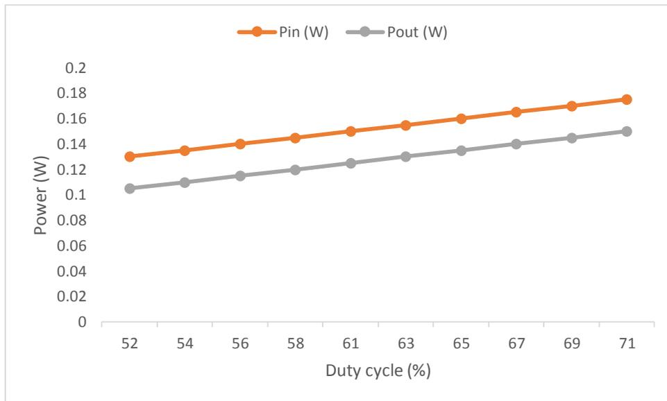
**Figure 8:** Efficiency of universal motor driver.
