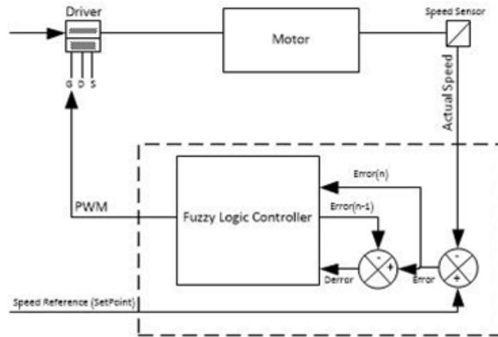
Figure 3: Controller diagram block.
