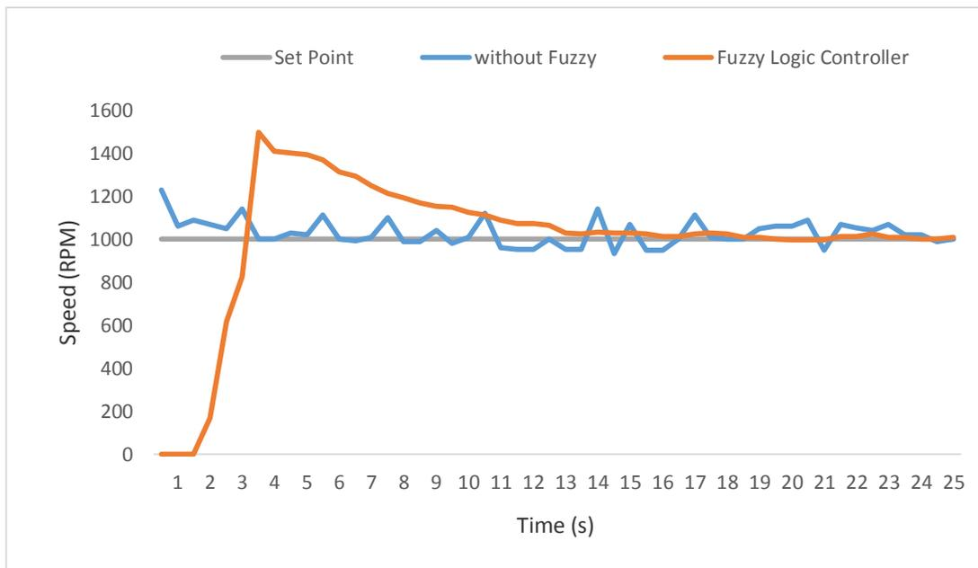
**Figure 9:** Speed testing without load condition.
