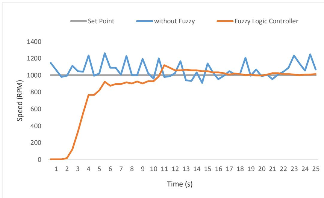
**Figure 10:** Speed testing loaded condition.
