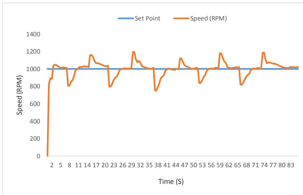
**Figure 11** : Speed testing results by raising the setpoint while loaded and load shedding conditions.
