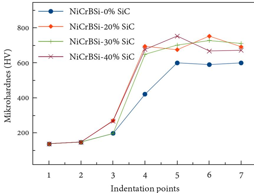
**Figure 6:** Hardness value is taken from the substrate (started at point 1) to the coating.
