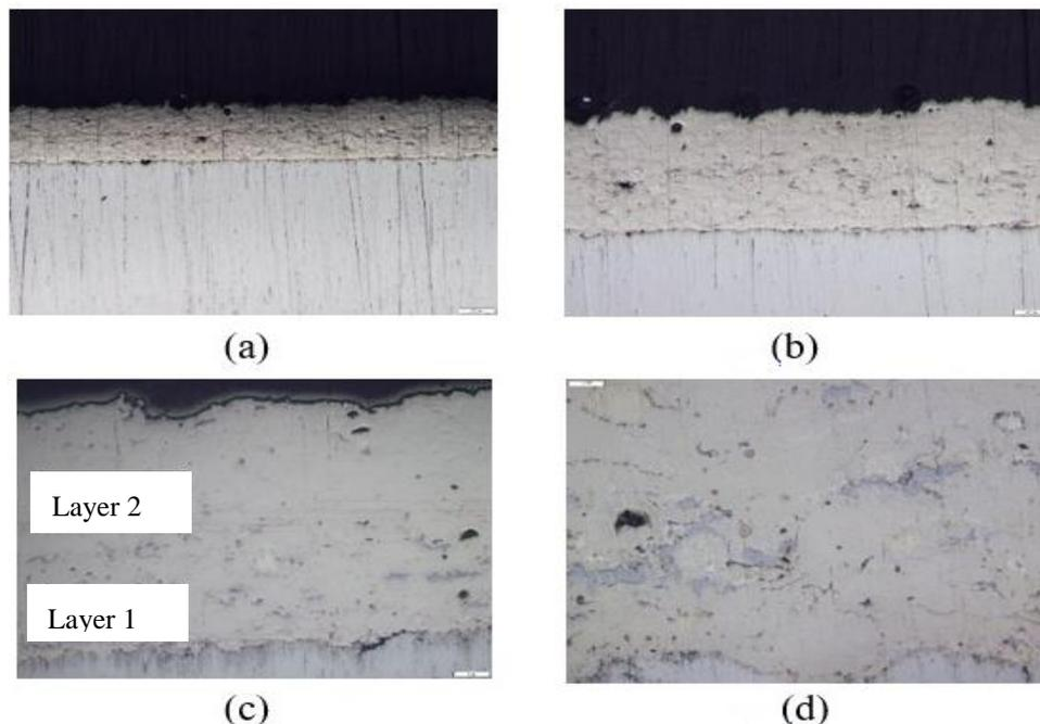
**Figure 1:** Microstructure of sample X (100% CrBSi) containing information about the thickness and microstructure of coating at several magnification; a) 50, (b) 100 X (c) 200 X (d) 500 X.
