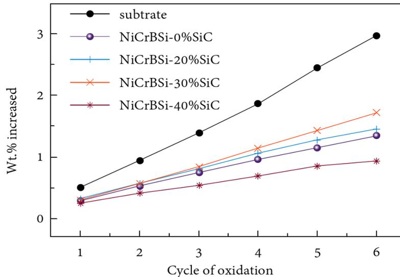
**Figure 7:** Thermal oxidation of sample as measured by weight gained during the cyclic measurement.
