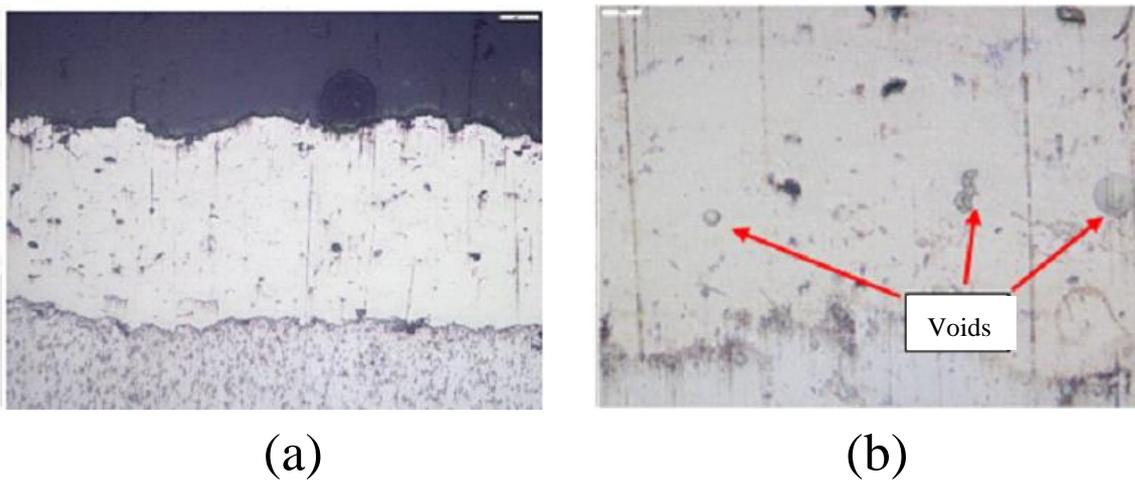
**Figure 3:** Microstructure of specimen B (70% NiCrBSi-30% SiC) at: a) 200X, (b) 500 X.
