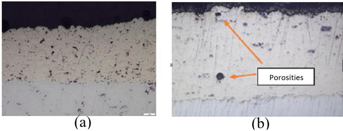
**Figure 2 :** Microstructure of Specimen A (80 % NiCrBSi-20% SiC) at: (a) 100 X, (b) 200 X.
