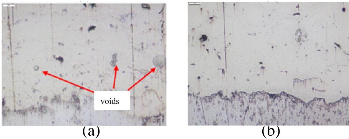
**Figure 4:** Microstructure of Specimen A (60 % NiCrBSi-40% SiC) at: (a) 200X, (b) 500 X.
