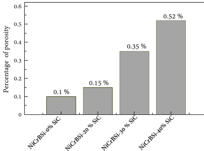
**Figure 5:** The effect of SiC fraction on amount of porosities.
