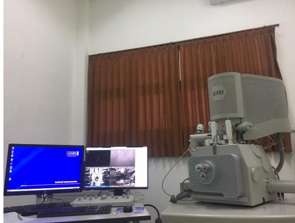
Gambar 4. Alat pengujian EDS ( energy Dispersive X-Ray Spectroscopy )
