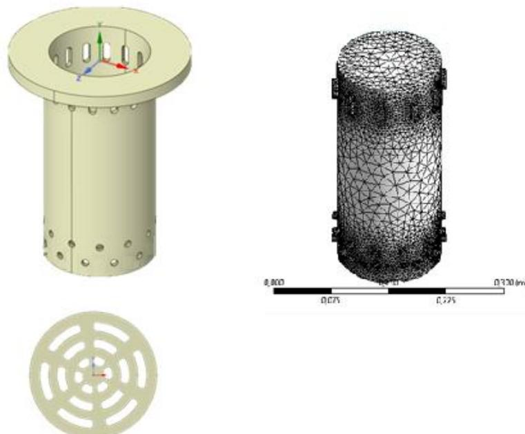
**Figure 4.** Geometry and the meshing of the burning chamber
