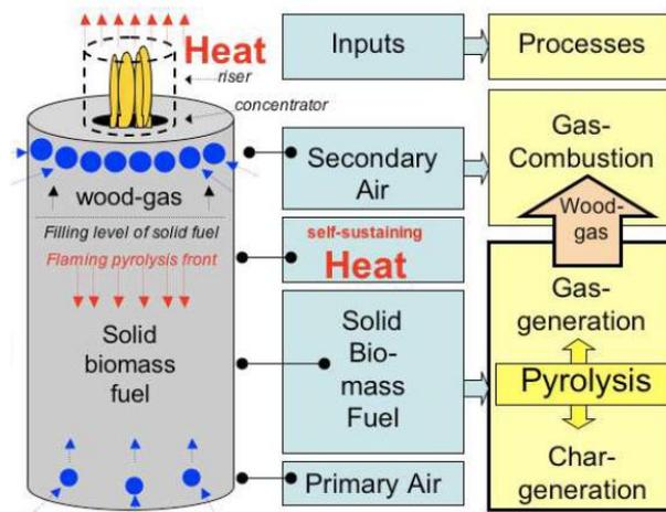
**Figure 1** Basic design of TLUD gasifier, Design: Roth [10]
