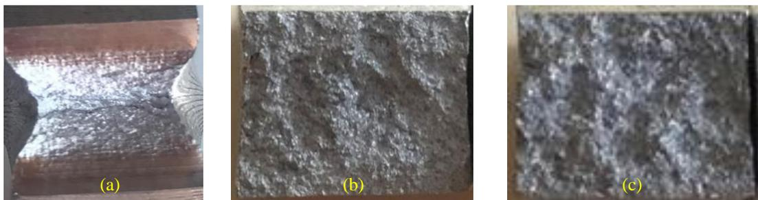
**Figure 8.** Fracture surface of specimens after impact test a) 0.12 % wt Fe, b) 0.16 % wt Fe, c) 0.20 % wt Fe
