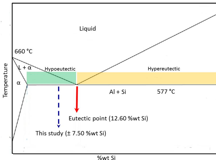
**Figure 1.** Al-Si phase diagram
