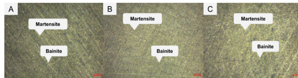
Figure 4. Metallographic Test Results of Quenching - Tempering Specimens (A) QT1 holding time 5 minutes, (B) QT2 holding time 15 minutes, (C) QT3 holding time 25 minutes (10 µm Scale)
