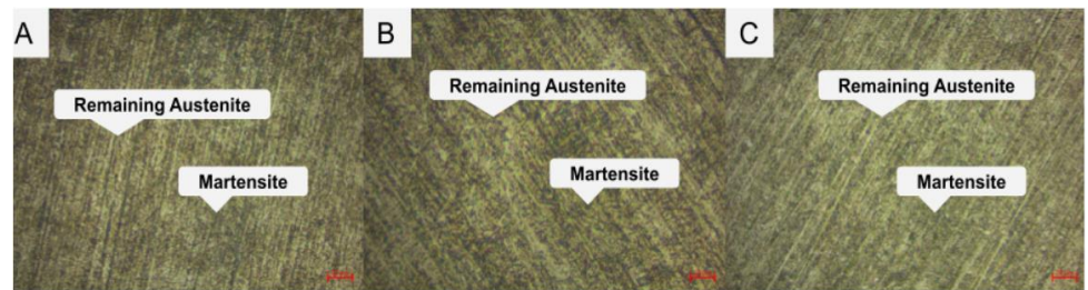
Figure 3. Metallographic Test Results of Quenching Specimens (A) Q1 5 min hold time, (B) Q2 15 min hold time, (C) Q3 25 min hold time (10 µm Scale)
