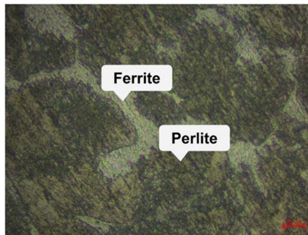
Figure 2. Metallographic Test Results of Untreated Specimens (10 μm Scale)
