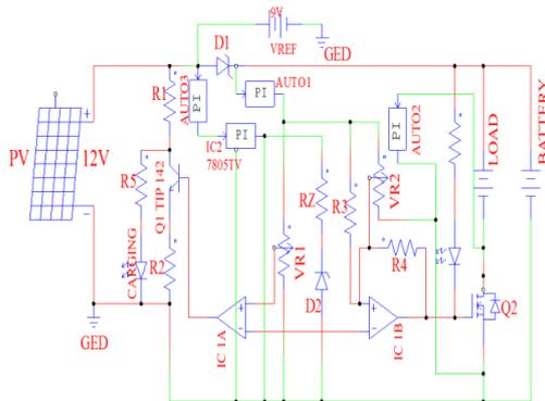
Figure 9. Charge Controller Circuit.
