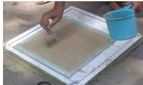
Fig. 2. Making samples of pineapple leaf fibre PMC with hand lay-up.
