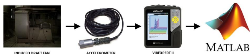
Figure 3. The processing scheme of vibration signal
