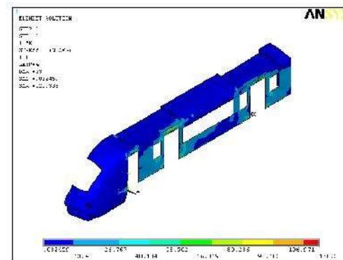
**Gambar 23** – Tegangan Von Mises Pada Layer 4 (Aluminium) Kasus 2
