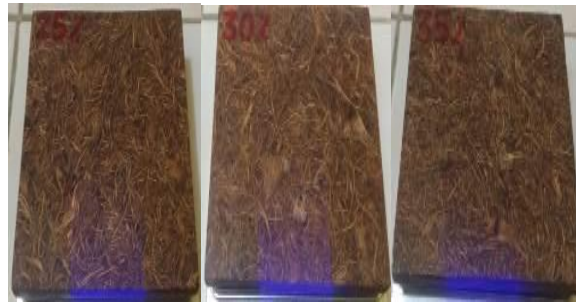
Figure 6. Partition boards with variations in weight fraction of 25%, 30%, and 35%.
