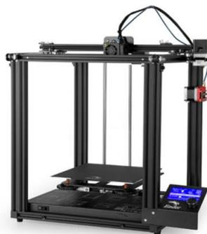
**Gambar 2:** Mesin 3D *printing* Ender 5 Pro
