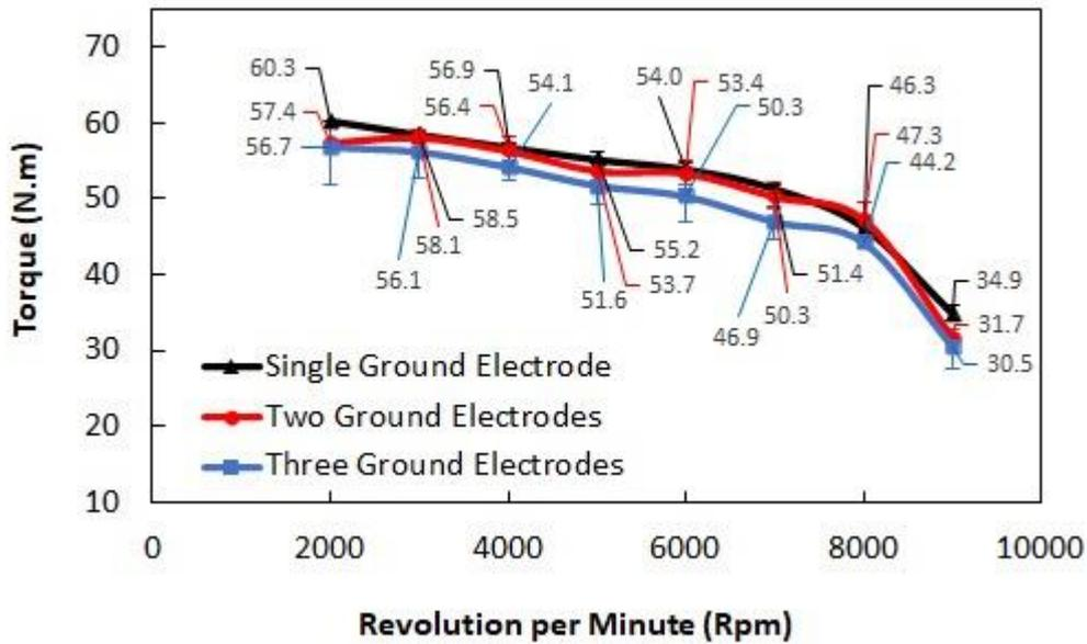
Figure 3. Graph of vehicle Torque as the function of angular velocity on the chassis dynamometer test.
