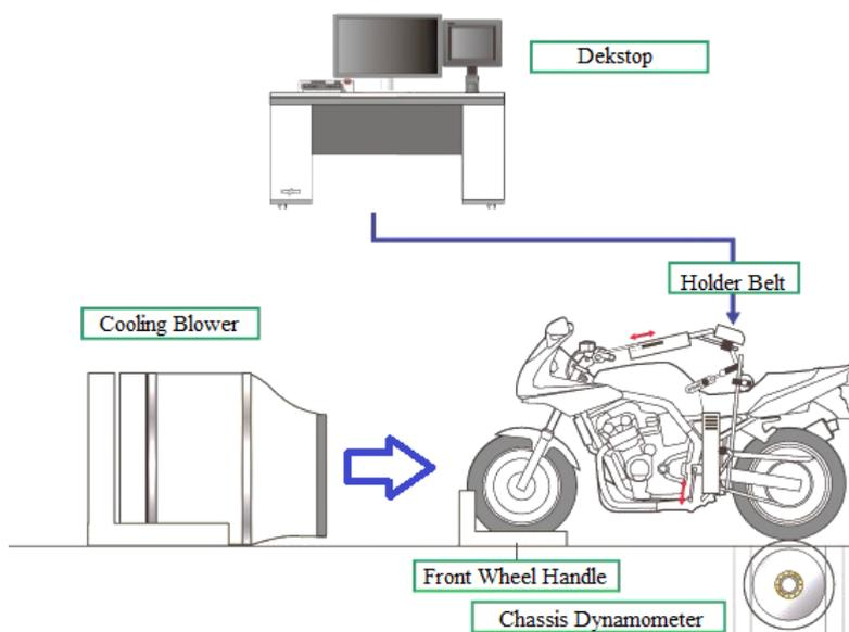
**Figure 1.** The data collection scheme uses a Chassis Dynamometer[24].
