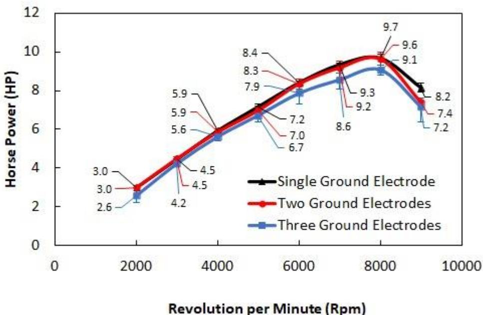
Figure 2. Graph of vehicle power as the function of angular velocity on the chassis dynamometer test.
