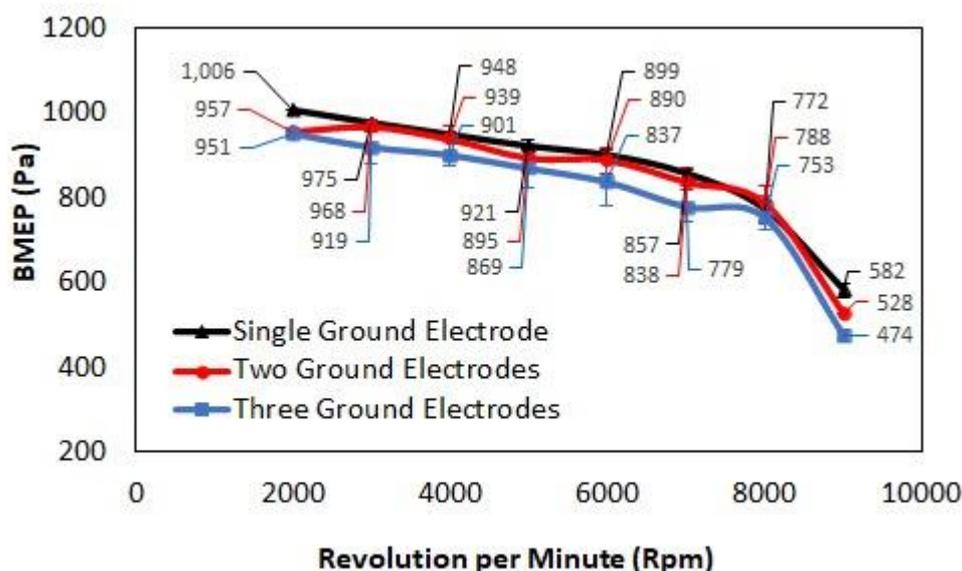
Figure 5. Graph of vehicle BMEP as the function of angular velocity on the chassis dynamometer test.
