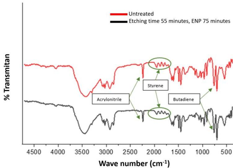
**Figure 3:** FTIR analysis of ABS.
