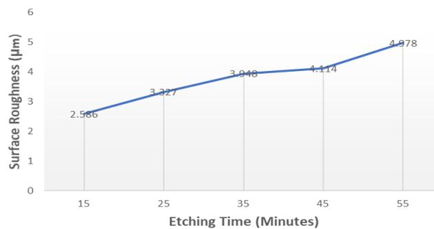
**Figure 1:** Relationship between etching time and ABS surface roughness.
