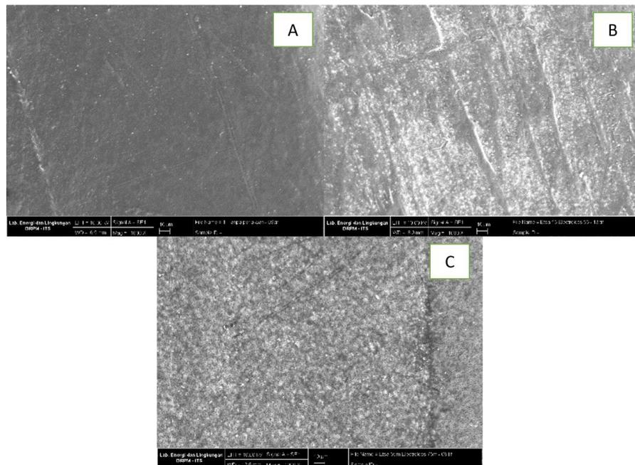
**Figure 4:** Surface of ABS (A) untreated (B) etching time 15 minutes ENP 55 minutes (C) etching time 55 minutes ENP
