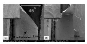
Fig. 7. SEM images of side view on as cast and partially crystallized Zr<sub>54</sub>Al<sub>17</sub>Co<sub>29</sub> BMG samples with 50% crystallinity. (Insets: fracture surface morphologies)
