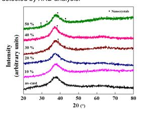
**Fig. 4.** XRD patterns of as cast and partially crystallized Zr<sub>54</sub>Al<sub>17</sub>Co<sub>29</sub> BMG samples with 10, 20, 30, 40, and 50% crystallinities.
