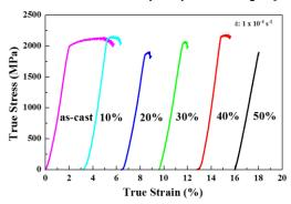
Fig. 6. True stress-strain curves of as cast and partially crystallized Zr<sub>54</sub>Al<sub>17</sub>Co<sub>29</sub> BMG samples with 10, 20, 30, 40, and 50% crystallinities.
