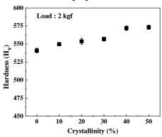
Fig. 5. Hardness of as cast and partially crystallized Zr<sub>54</sub>Al<sub>17</sub>Co<sub>29</sub> BMG samples with 10, 20, 30, 40, and 50% crystallinities.
